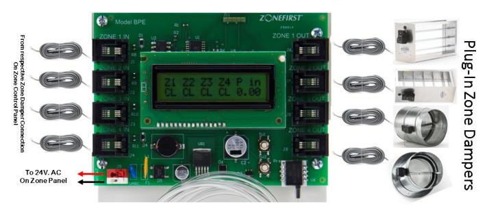
NOTE: If there is a specific zone that should not be used to relieve air, wire zone damper directly to zone panel.
