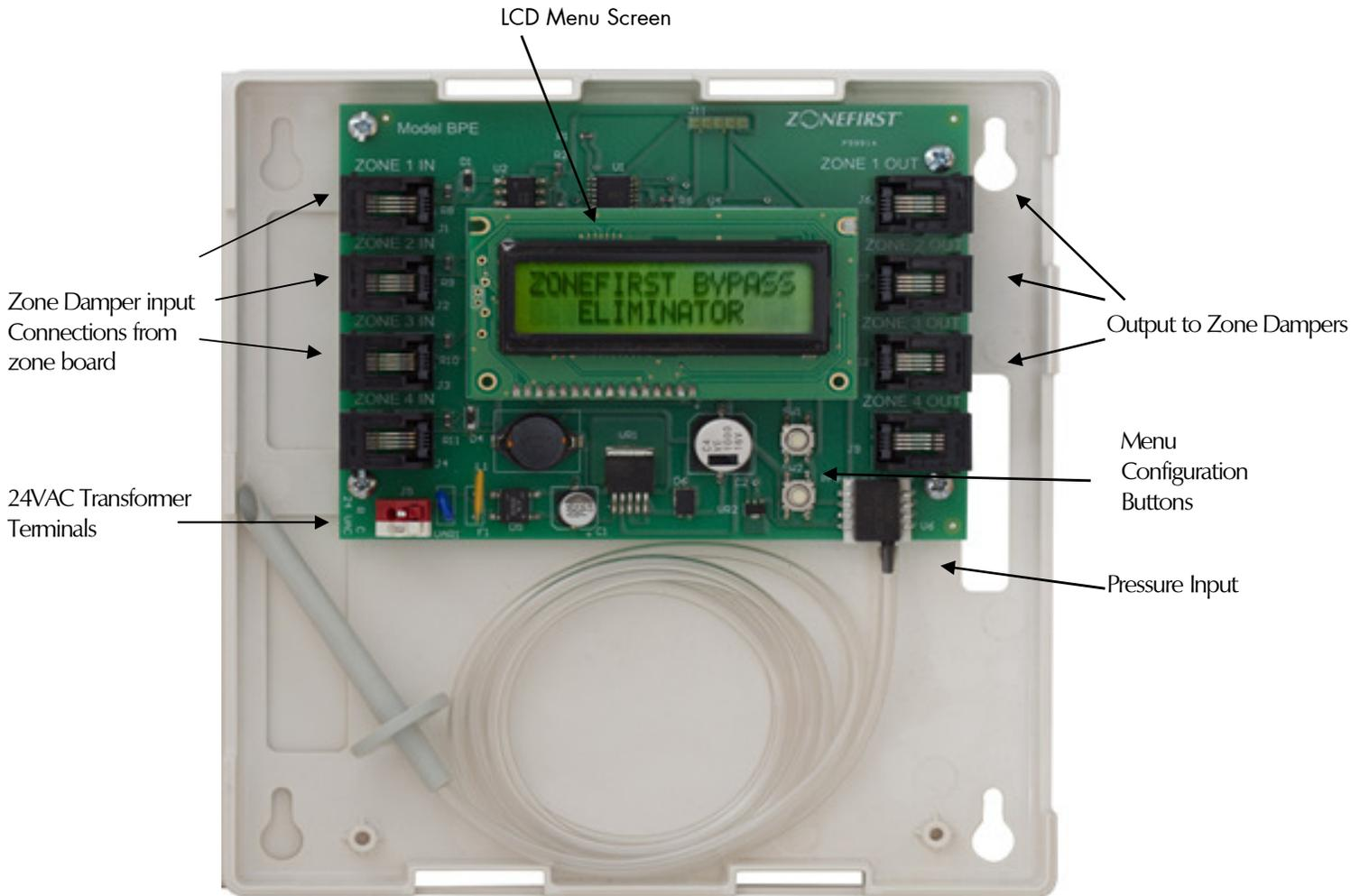
The Bypass Eliminator™ (Model BPE) Control is an interface between a ZONEFIRST Zone Control Panel and its zone dampers. The BPE is used to eliminate the need for a traditional separate by-pass duct and damper directed back into the return duct. The BPE can **ONLY** be used with ZONEFIRST'S Plug-In Zone Dampers and control panels.
