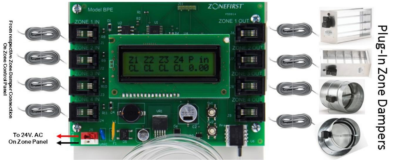
NOTE: If there is a specific zone that should not be used to relieve air, wire zone damper directly to zone panel.
