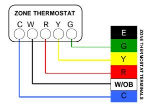
WIRING DIAGRAM 2 - Heat Pump Thermostat
