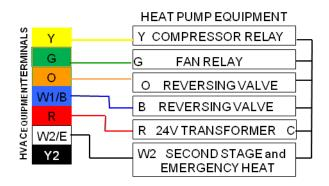
WIRING DIAGRAM 6 – Two Speed Compressor Heat Pump
