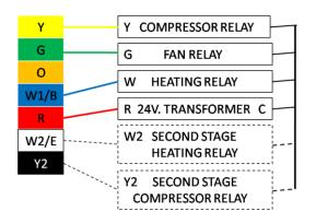
WIRING DIAGRAM 5 - Single Speed Compressor Heat Pump
