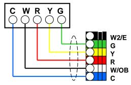
WIRING DIAGRAM 2 — Heat Pump Thermostat
