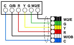
WIRING DIAGRAM 3 - HVAC Equipment - Conventional Single Stage and Two-Stage Equipment
